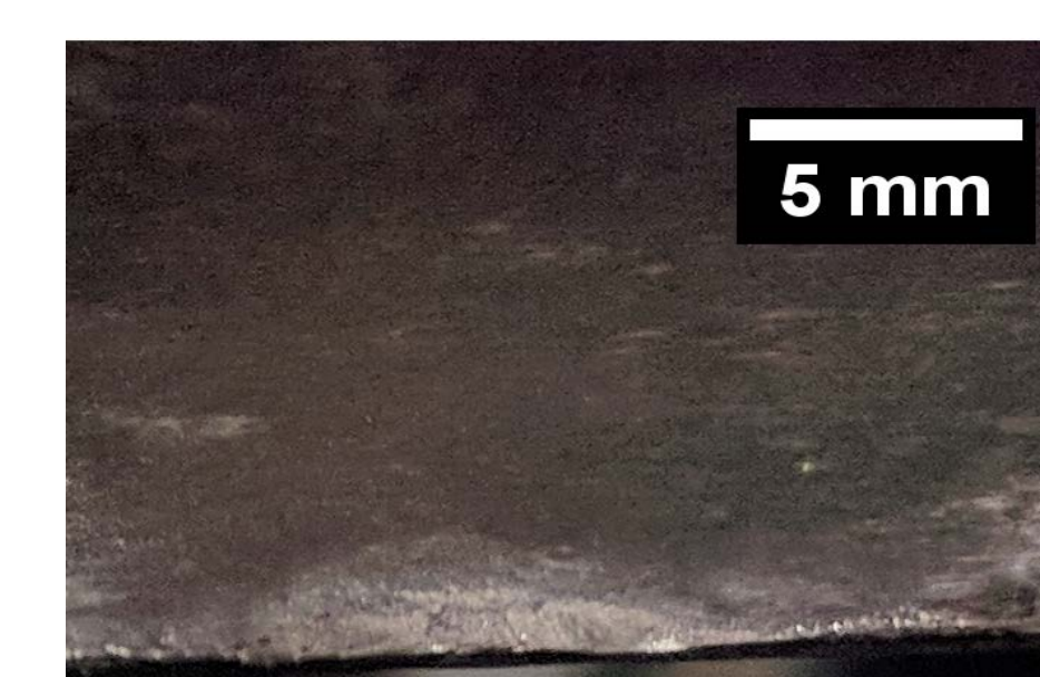
Figure 9: Smeared sliver on sample from coarse debris lost during rolling.
